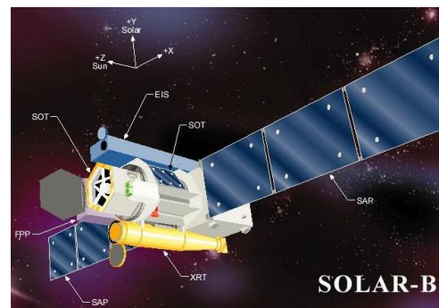
Figure 1. Schematic of the Solar-B satellite showing the locations of the instruments; SOT is the Solar Optical Telescope which will produce high-quality vector magnetograms of active regions.
